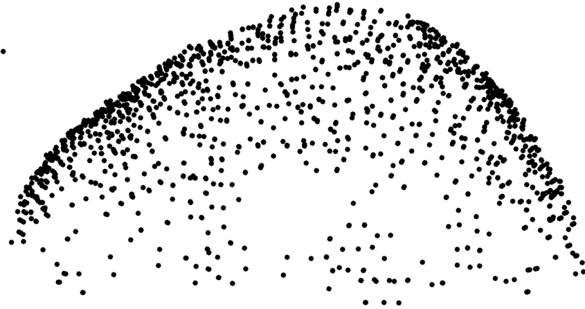
Figure 11: The ultrasound-derived point cloud from the surface of a 3D-printed PVA skull model showing the point cloud reconstruction method qualitatively looks successful.
